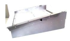
A pair of 19" rack ears is provided with the **PA12**. The ears replace the front and side trims so that the console can be mounted in a rack, plinth or case. Note that the PA12 can fit into a standard 19" rack. The ears can fit in one of two positions depending on how you want to mount the console in the rack or other furniture.
